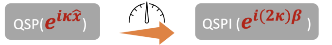
FIG. 3. Pictorial illustration of how in the bosonic QSP interferometric protocol, the qubit measurement enacts a duality between a polynomial transformation on the bosonic quadrature operators and a polynomial transformation on the sensing parameter \beta via QSPI.
